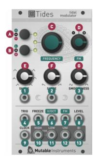
**A. Mode switch**. This button cycles back and forth between Tides' 3 operation modes: AD envelope (green LED), cyclic (LED off) and AR envelope (red LED). Note that a trigger pulse (or gate) must be sent to the TRIG input for the AD envelope (or AR envelope) to be triggered!
