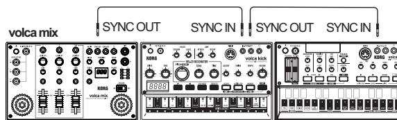
In order to start the sequencers of chained volcas all at once, first arm the sequencers by pressing the ▶(play) button on the connected volcas, then press the ▶(play) button on the volca mix.
