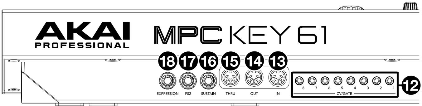
12. **CV/Gate Out** (1/8" / 3.5 mm, TS): MPC Key 61 will send control voltage (CV) and/or Gate signals over these outputs to optional external synths or sequencers. Use standard 1/8" (3.5 mm) TS cables to send a single CV/Gate signal per output.
