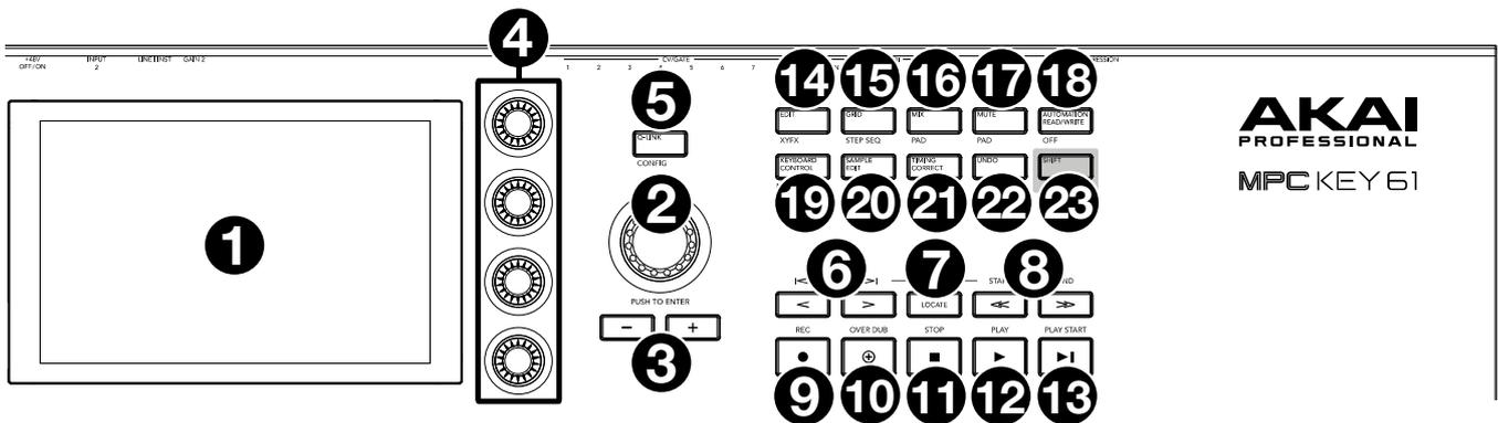
1. **Display:** This full-color multi-touch display shows information relevant to MPC Key 61's current operation. Touch the display (and use the hardware controls) to control the MPC interface. See the previous [Touchscreens](#) section to learn how to use some basic functions.
