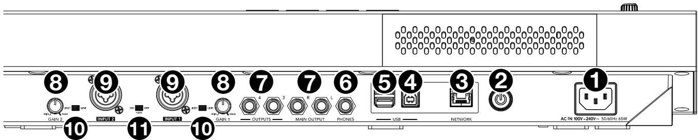
1. **Power Input:** Use the included power adapter to connect MPC Key 61 to a power outlet.
