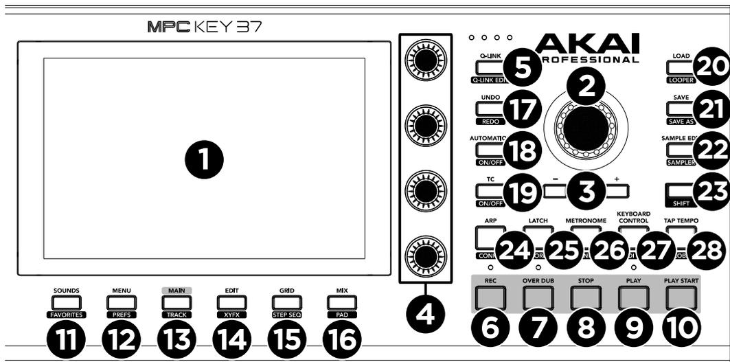
1. **Display:** This full-color multi-touch display shows information relevant to MPC Key 37's current operation. Touch the display (and use the hardware controls) to control the MPC interface. See the previous [Touchscreens](#) section to learn how to use some basic functions.
