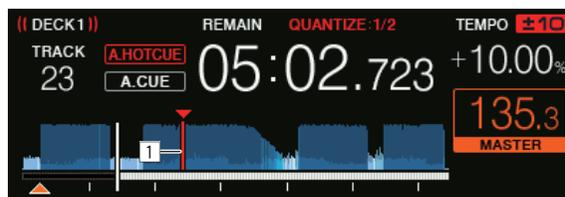
When the playback position reaches to the setting point, the loop is set automatically and loop playback begins.
