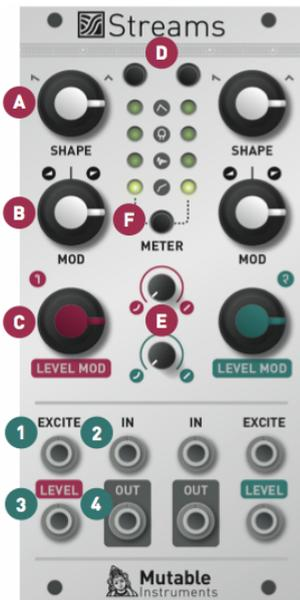
**A. Channel envelope shape.** This knob controls the overall attack and decay characteristics of the selected function - for example envelope times, and vactrol or envelope followers reaction time.
