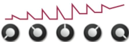
The **MOD** knob controls how the brightness (filter cutoff frequency) is affected by the envelope. Starting from the minimum setting, turning the knob clockwise will progressively increase the amount of envelope modulation on the brightness - with the maximum amount reached when the knob is at noon. Then, turning the knob will reduce the envelope amount, but will compensate by adding an offset. Thus, at 7
